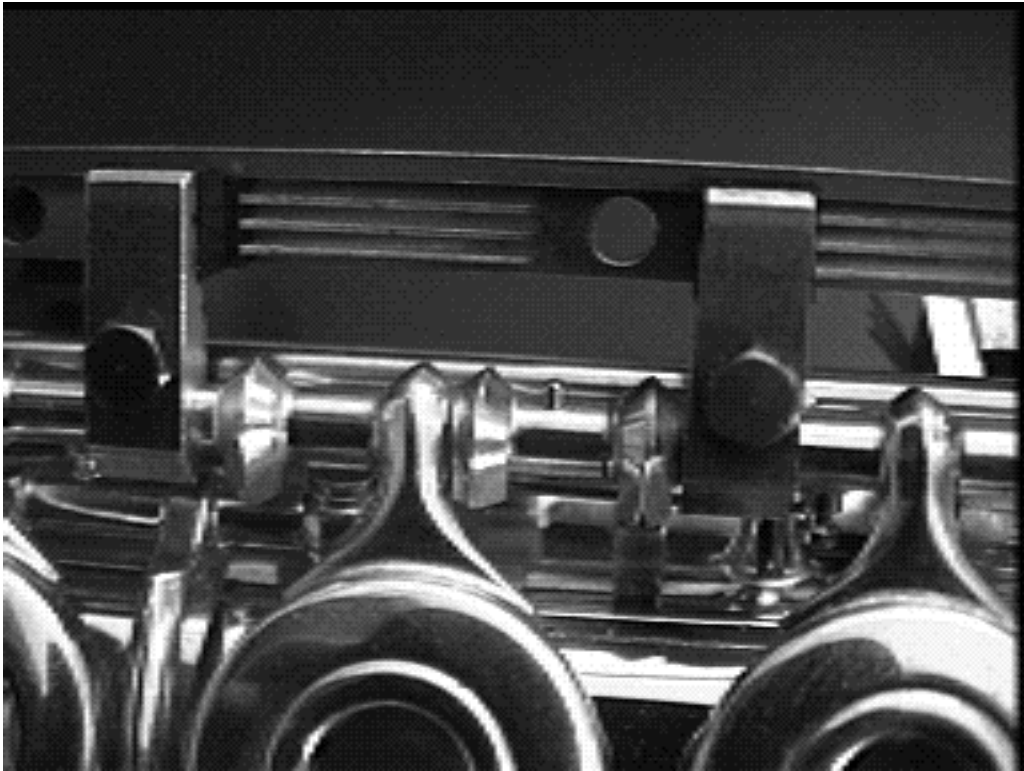
Figure 7.15: Close view of the fixation system of the magnets connected to the key-pad bar.
